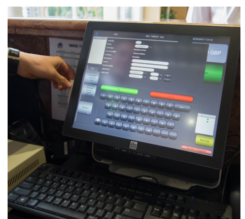
Parking can be validated in four ways - at the Paystation, with the POS at Receptions (right), with the Validator (top right) and with Whitelists.
